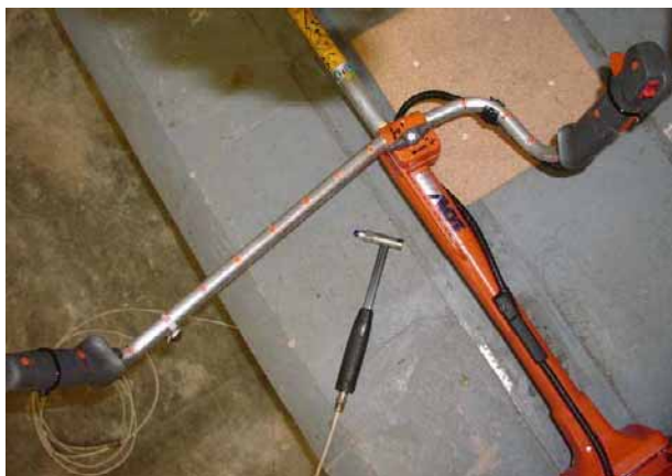
Figure 15: Nodal points on cow-horn handle
