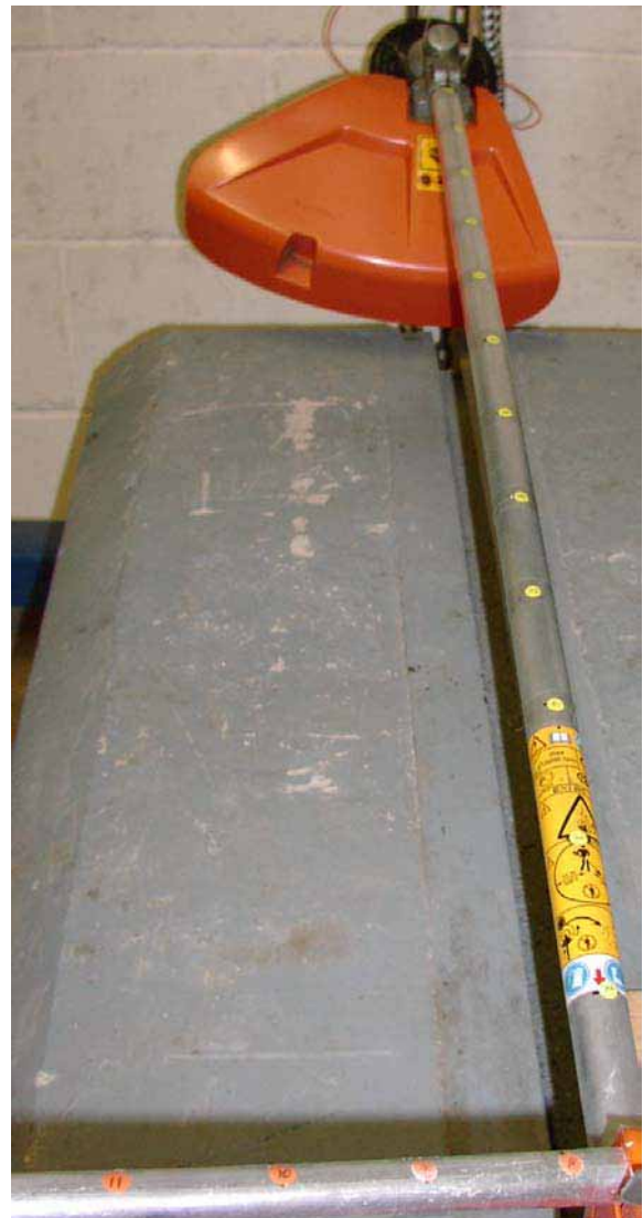
Figure 16: Nodal points on shaft (some points on cow-horn handle also shown)
