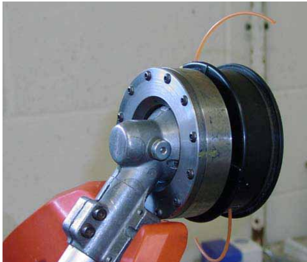
Figure 9: Experimental auto-balancer fitted behind cutting head
