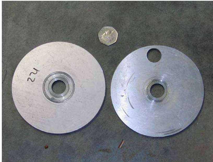
Figure B3: Artificial discs, “balanced” and with 5gm unbalance
