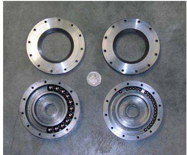
Figure 11: Components of experimental auto-balancer – Left, 6mm balls; Right, 12mm balls
