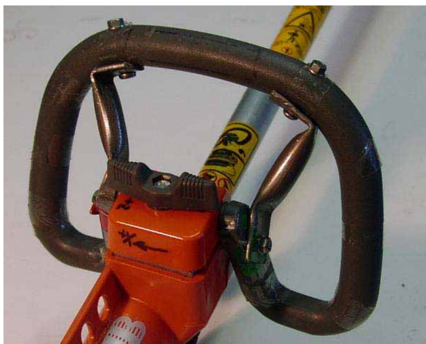
Figure 24: Loop handle with added stiffness.
