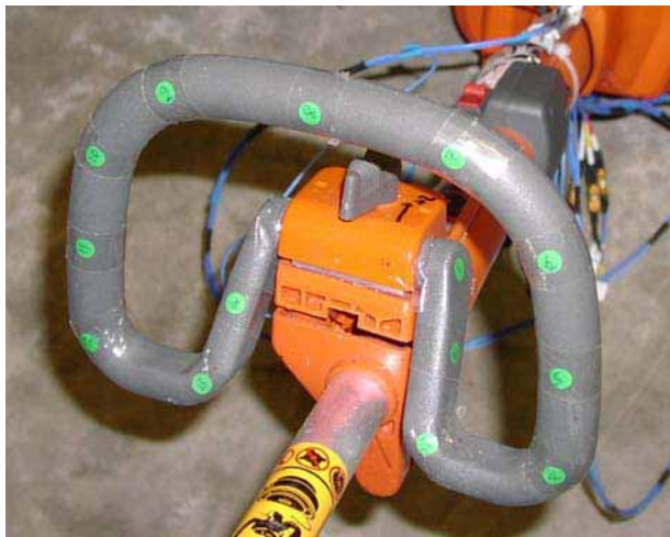
Figure 14: Nodal points on loop handle
