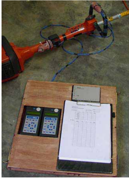
Figure B1 Loop handle machine showing Measuring equipment
