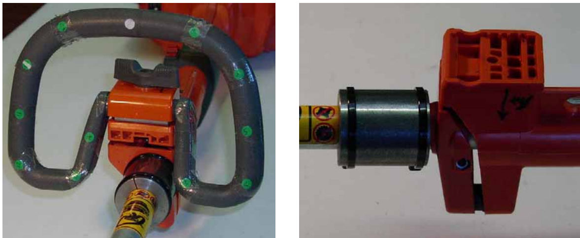
Figure 23: Mass loading to increase shaft impedance at mounting bracket.
