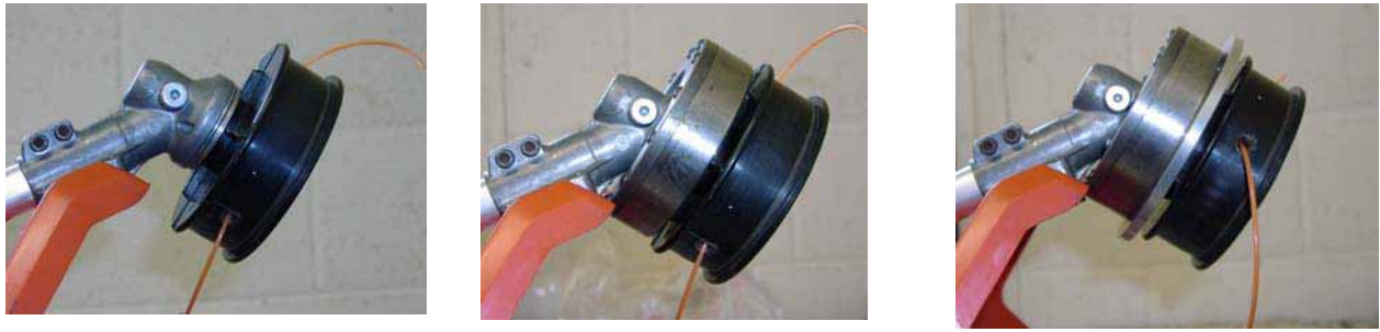
Figure 12: Head arrangements: Left – standard, Centre – with balancer; Right – also with artificial unbalanced disc
